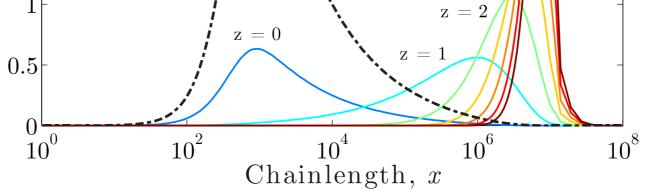
GPC chain length distributions at the gel point obtained in each radical class z are shown as solid lines. The values of the overall distribution, depicted by a dashed line, are scaled by a factor 4 for comparison
